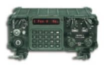
**PANTHER V**50 watt vehicle/base station radio
